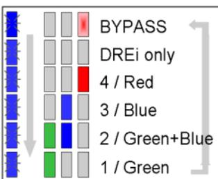
A sequence starts with the *DREi Micro* on Standby bypassing the audio signal from input to output, so you will be hearing your equipment without the DREi process. After 10 seconds it auto connects the *DREi Micro* with SCENE OFF (DREi process only). After another 10 sec. it will change to Red SCENE, and then to the other SCENES. After Green it will return to Standby and start a new cycle.
